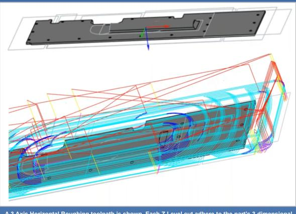
A 3 Axis Horizontal Roughing toolpath is shown. Each Z Level cut adhere to the part's 3 dimensional shape, tolerance, stock allowance, cut parameters and cut level controls.
