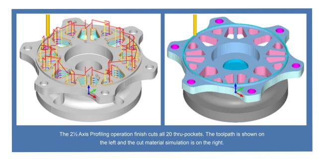
This completes the top side for this part. The Setup1 as shown in the Machining Job tree above can be posted out in one g-code file (if you have an automatic tool changer) or posted out as separate g-code files, one operation at a time if you need to change tools manually for each operation.
