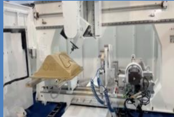
Here is a 5-axis component being machined on Dovetailors 5-axis Machining Center
