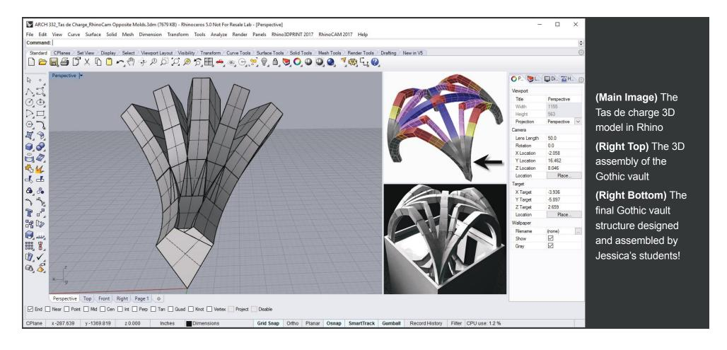
In the Rhino display above we see the Tas de charge 3D model and its position within the Gothic Ribbed Vault structure. In vaulting architecture, the Tas de charge is the key component that supports the weight of the structure. In the Rhino display below we see how the part is used to model the upper and lower cavity halves of a mold used to cast the part.
