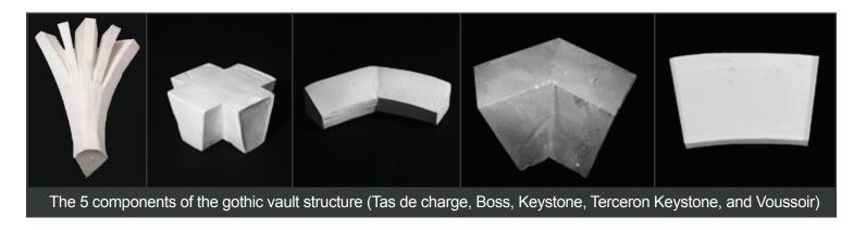
Here are the 5 components of the vault structure from left to right (Tas de charge, Boss, Keystone, Terceron Keystone, and Voussoir). While this is a group project, each student has access to the actual Rhino parts and assembly for 3D modeling and RhinoCAM for programming toolpaths on the school's 3 Axis Techno CNC machining center. Since the Tas de charge is the most complicated piece, we have selected it for further discussion below.
