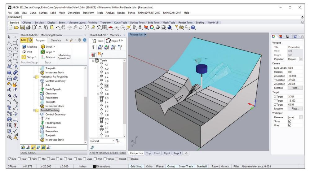
The RhinoCAM plugin is loaded showing the Machining Browser, Machining Objects Browser with Tool Library and the 3 Axis Parallel Finishing toolpath simulation for the lower cavity of the Tas de charge mold.
