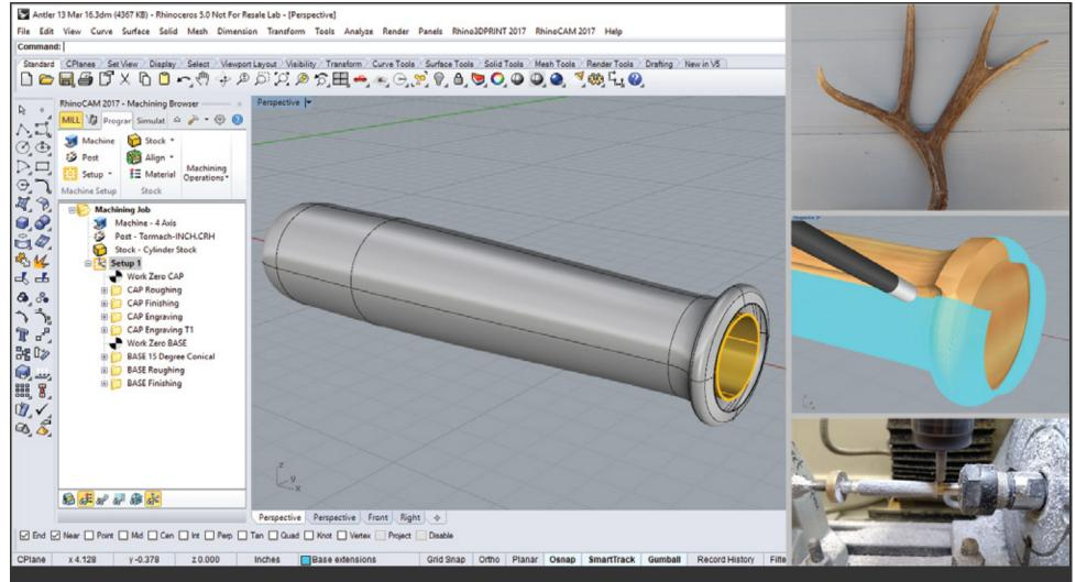
Here we see the Antler Pen Base with brass sleeve insert modeled in Rhino 5.0. On the left we see the RhinoCAM Machining Browser showing the 4 Axis Setup. (Inset Top Right) The actual Elk antler stock is shown. (Inset Middle Right) The 4 Axis Parallel Finishing operation is being simulated in RhinoCAM. (Inset Bottom Right) The 4 Axis Parallel Finishing toolpath is shown being cut on the Tormach 4 Axis machining center.
