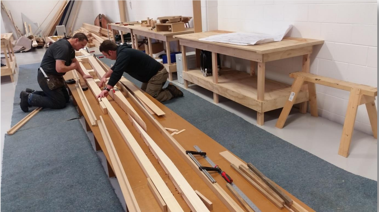
Assembling the wing spars
