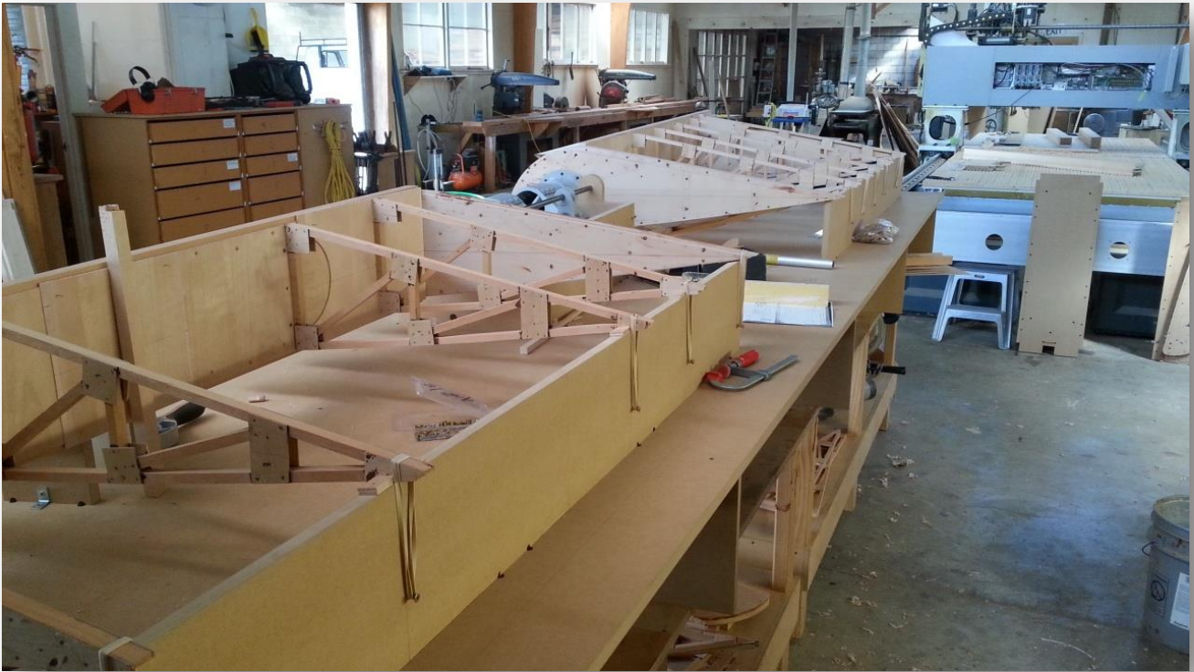
The Ailerons during the assembly process
