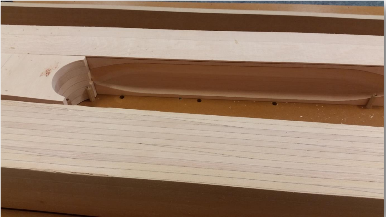
The assembled wing spar on jig.
