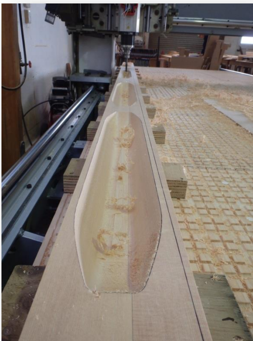
CNC machining of wing spar recesses
