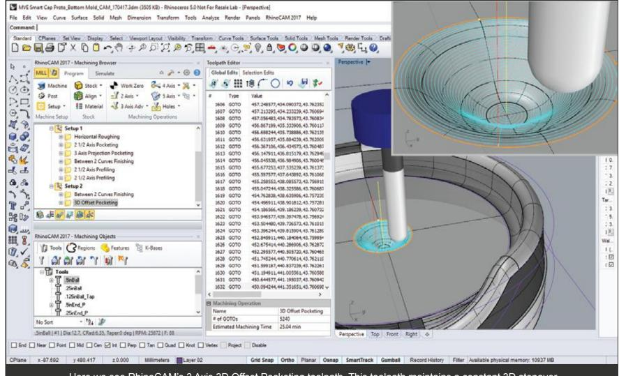
Here we see RhinoCAM's 3 Axis 3D Offset Pocketing toolpath. This toolpath maintains a constant 3D stepover distance regardless of the topology of the part surfaces. This toolpath is excellent for contoured surface machining because of the very high-quality finish that can be achieved.
