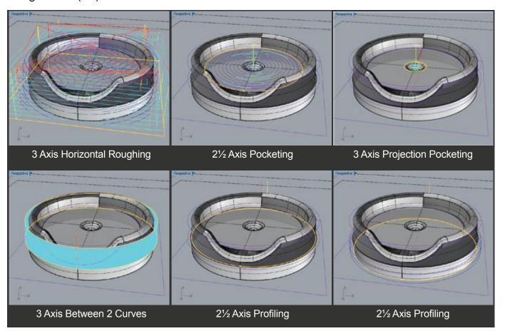
Here are the toolpaths in Setup 2 that Gordon has programmed using a 12.7 (1/2") ball mill:
