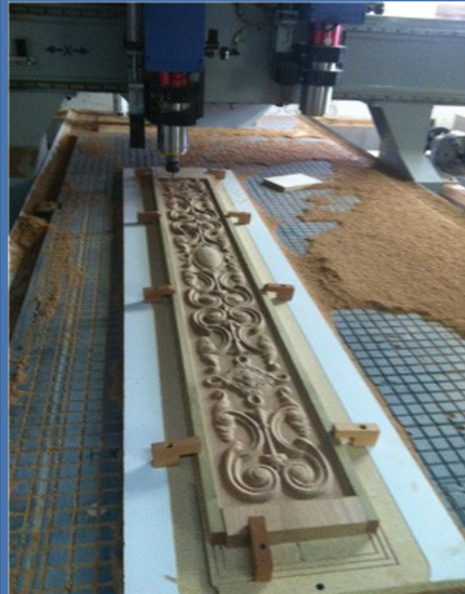
Actual panel relief being machined from RhinoCAM toolpaths on Jim's NewCNC3 Axis router.
