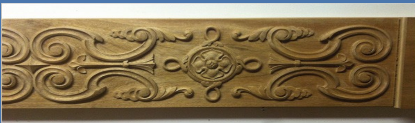
Actual Relief Machined with RhinoCAM toolpaths
