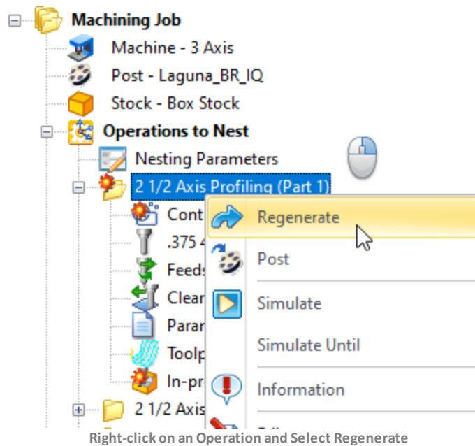
The toolpath is now generated with the modified settings. Notice that the In-process Stock is still flagged. This alerts you that it has not been simulated yet.
