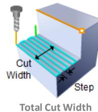
This will determine the stepover for each cutting pass beginning at your total cut width and ending at your control geometry.
