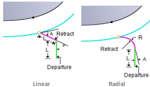
For the **Departure Motion**, enter the departure **Length (L)**. Then, depending on the stock material and cut pattern select the departure angle as either **Normal**, **Tangent** or **Specify Angle (A)** with respect to the stock.
