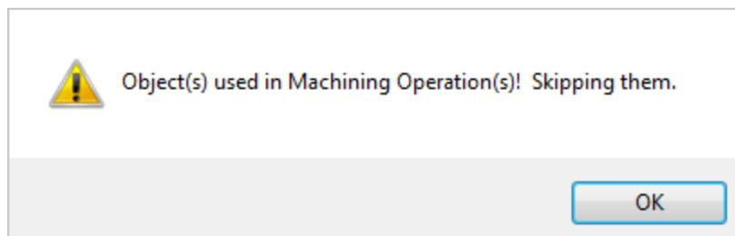
This error can occur when attempting to delete a tool that is currently associated with machining operation:
