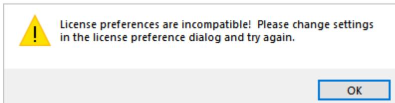
If [Using Lan Daemon](#) is checked and you are entering a valid node locked activation code in the license dialog, the following message is displayed. Make sure [Using Lan Daemon](#) is unchecked before activating a node-locked license.
