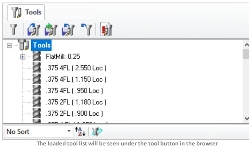
4. To perform the [Edit](#), [Rename](#), [Cut](#), [Copy](#) or [Paste](#) operations on any of these tools, hit the right mouse button while highlighting the desired tool.
