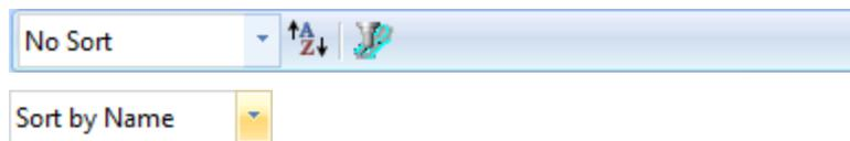
**Sorting Selector:** This allows you to sort the tool list. You can select **No Sort** or sort by Name, Number, Type and Diameter.
