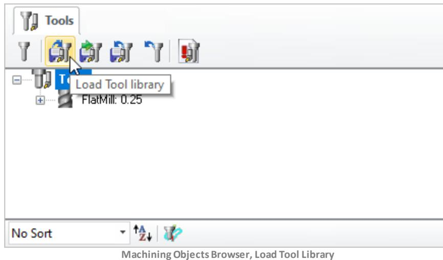
2. Browse to the folder, double click on the desired file to load it into [Profile-NEST](#) module. The folder of the last loaded tool library is displayed by default.
