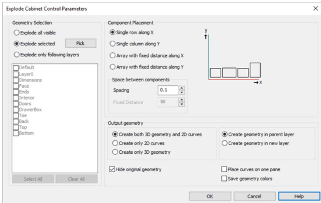
Dialog Box: Component Decomposition Control Parameters
