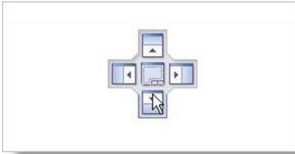
**For example:** Selecting the button on the widget with arrow pointing downwards on and releasing the left mouse button docks the selected browser below the specified browser.
