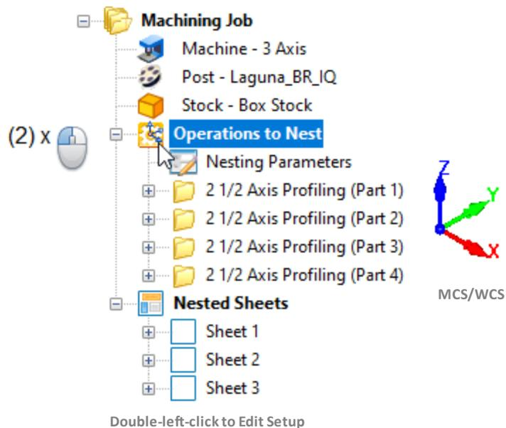
Editing an **Operations to Nest Setup (MCS)** displays the **Setup** dialog. This dialog allows you to modify that **Setup** orientation.
