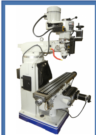
The CNC Masters Supra knee mill
