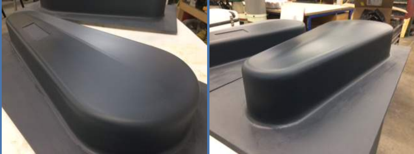
The two mandolin case core molds are shown. The case top is on the left and the bottom is on the right.
