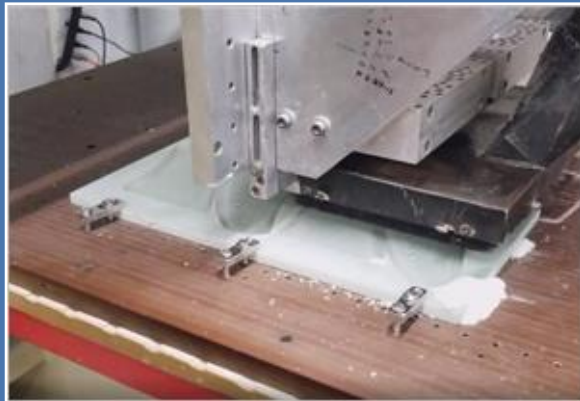
(K) Here we see Michael's Centroid-driven CNC router cutting a set of prototype wave fins from G-10 composite stock material.
