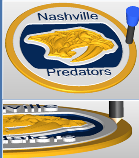
The resulting cut material simulation of all toolpath strategies in Setup 1 for the Predators® casted core.
