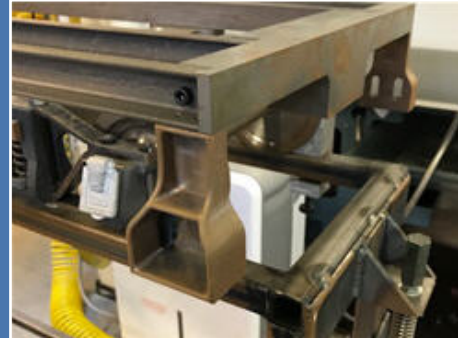
Tinder steps mounted on the Heisler coal car chassis.
