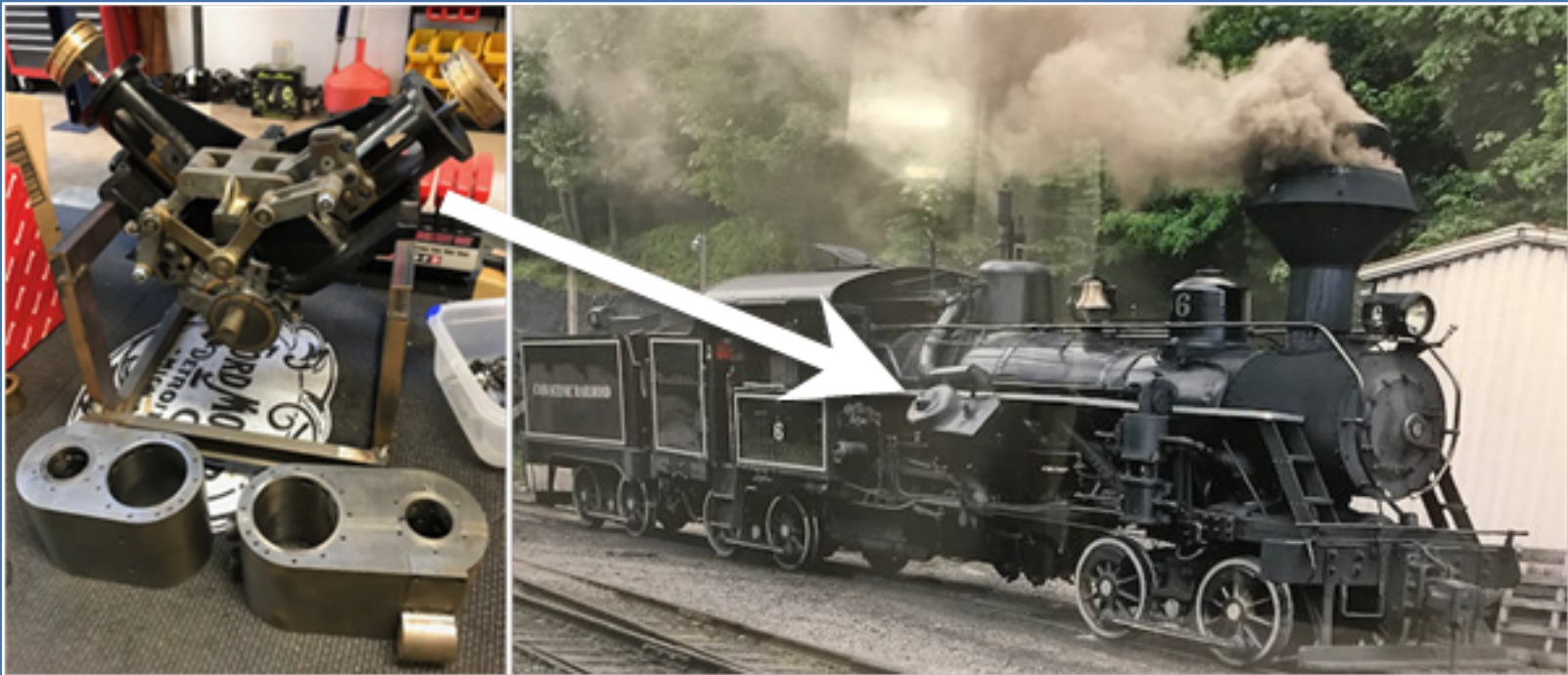
(Left) The 1/8 scale Heisler V2 engine replica under construction in Rex's shop. (Right) The Heisler engine #6 in action at the Cass Scenic Railroad, Elkins, WV.
