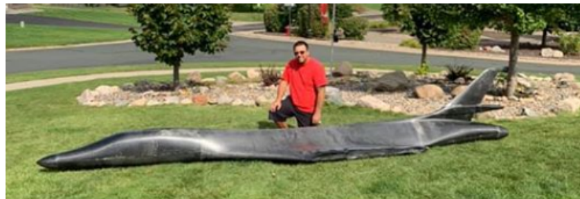
Zach and the 18 foot long RC B1 Lancer carbon fiber composite fuselage
