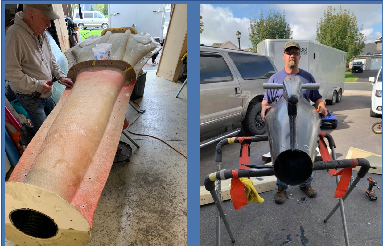
Richard Steine (Left) and Darren Bitzer (Right) assist with construction and assembly of the giant 18 foot long B1 Lancer carbon fiber fuselage.
