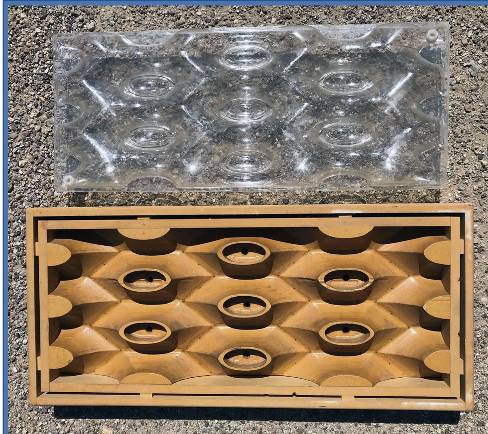
Here is another full size view of the vacuum form along with an actual hydro-container produced from recycled plastic.
