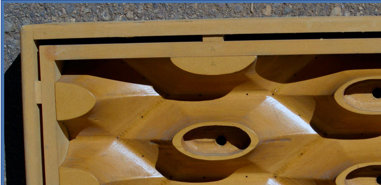
Here is a closeup of one of the the vacuum forms machined from RhinoCAM toolpaths.
