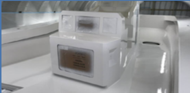
(C) Typical Bridge Console after Final Top Coat
