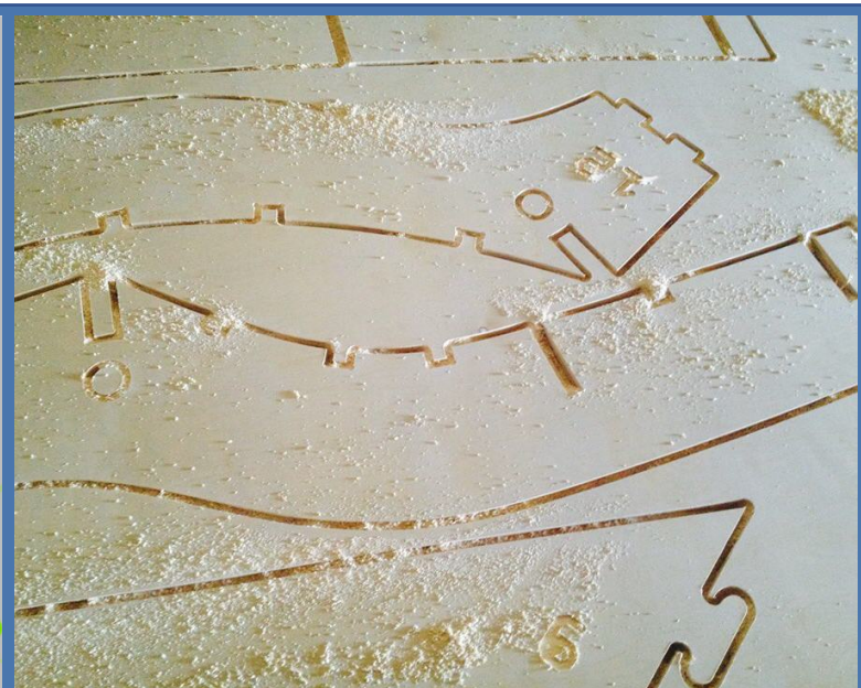
(B) The nested sheet of jig framing cut from RhinoCAM Toolpaths
