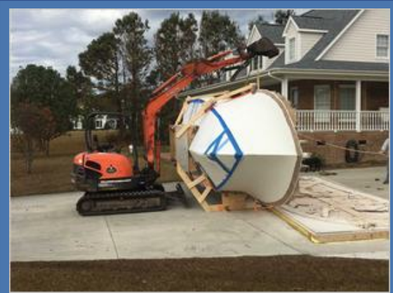
(E) The jig framing and completed outer hull is then turned right side up.
