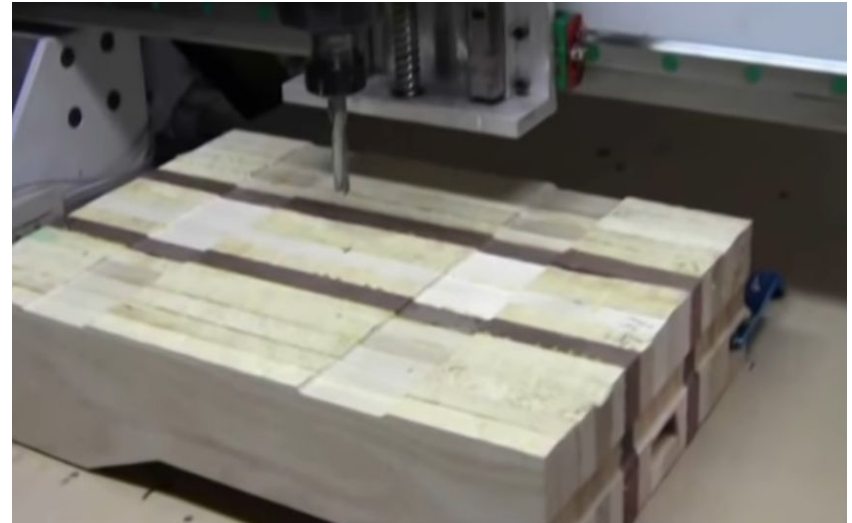
(B) The stock blanks are glued together and mounted to the CNC router bed.
