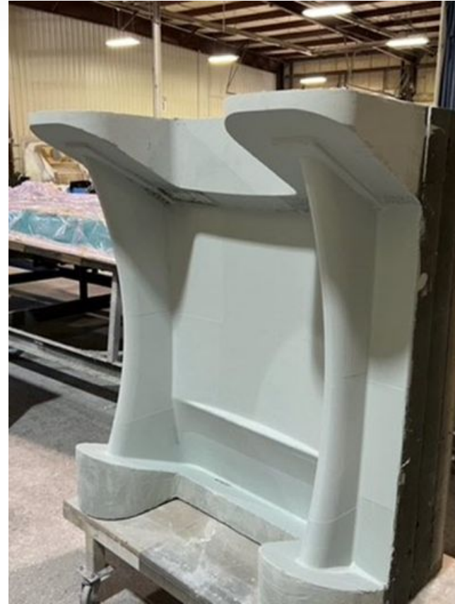
The finished core plug, one of several that are ready for layup.
