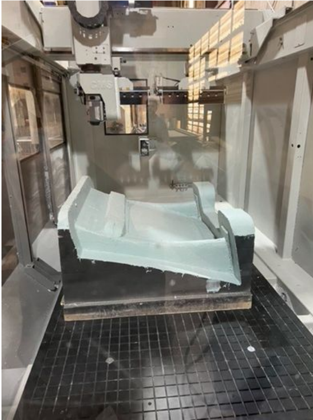
The core plug is still in the CMS Athena 5 Axis Machining Center.
